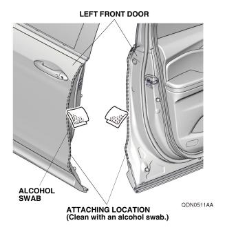
Close the left front and rear doors. Using a spray bottle with 3M protective tape application solution, spray the area where the left front door edge film will attach.
