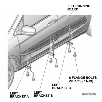
5. Tighten the six flange bolts loosely installed in step 3. Torque the flange bolts to 20 lb-ft (27 N⋅m).
