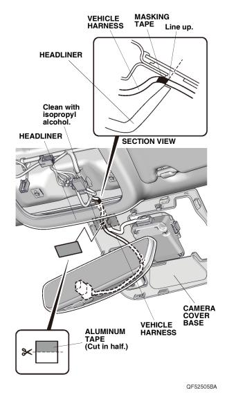
11. Using scissors, cut one aluminum tape in half. Line up the masking tape on the vehicle harness with the edge of the headliner, and secure the vehicle harness to the camera cover base with one half of aluminum tape.
