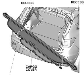
First, insert the left end of the cargo cover into the left recess. Then, compress the cargo cover, and install the right end into the right recess.
