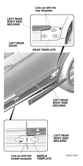
12. While applying light pressure against the left rear body side molding, carefully remove the taped adhesive backings.
