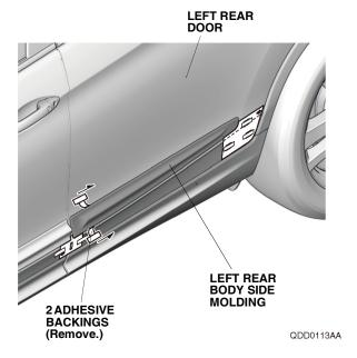
13. Using a rubber roller, apply firm pressure against the left rear body side molding and roll from one end to the other. Apply firm pressure especially at the ends.
