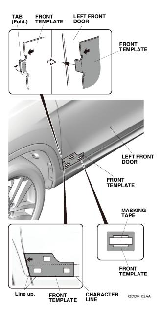
2. Line up the middle template with the character line, and attach it to the left front door and left rear door with strips of masking tape as shown.
