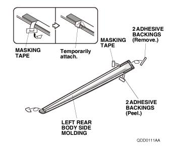
11. Line up the left rear body side molding with the middle and rear templates, and attach it to the left rear door as shown.
