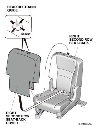
Secure the right second row seat-back cover with the fasteners.
