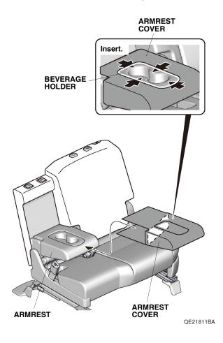
12. Raise the armrest. Pull out the armrest cover between the armrest and left second row seat-back, and secure the armrest cover with the fasteners.
