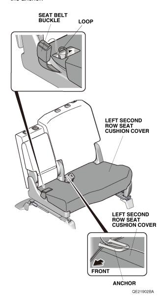
16. Secure the left second row seat cushion cover with the fasteners.
