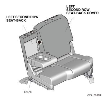
Secure the left second row seat-back cover with the fasteners.
