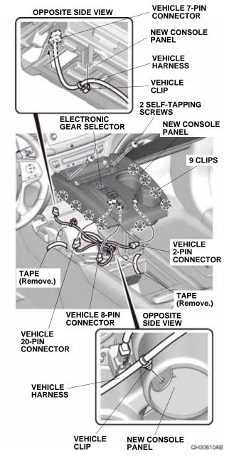
11. Install the new console panel with nine clips and two self-tapping screws removed in step 3.
