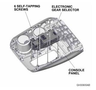
5. Install the electronic gear selector to the new console panel with six self-tapping screws removed in step 4.
