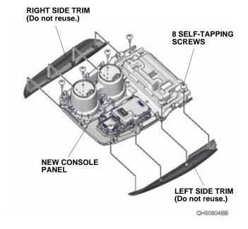
8. Install the left and right side trim panels to the new console panel with eight self-tapping screws removed in step 6 or 7. Go to step 10.
