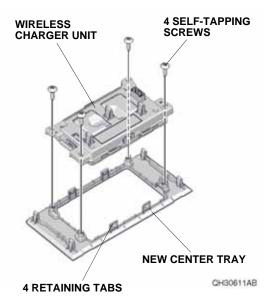
13. Plug the vehicle 7-pin connector into the wireless charger unit, and install the new center tray to the new console panel with four clips.
