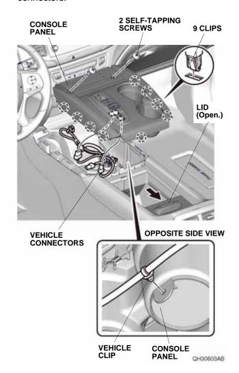
4. Remove the electronic gear selector from the console panel removed in step 3.
