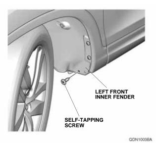
4. Loosely secure the left front splash guard on the left front inner fender with two 5 x 20 mm self-tapping screws and the self-tapping screw removed in step 3.
