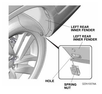
Loosely install the left rear splash guard to the rear bumper and left rear inner fender with two 5 x 20 mm self-tapping screws and the two self-tapping screws removed in step 7.
