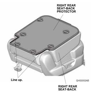
24. Lift the right rear seat-back protector, and attach masking tape to the right rear seat-back where the snaps will be located.
