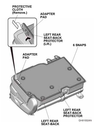
17. Apply pressure to the left rear seat-back protector at the area were the hook and loop is located, make front to back movements while applying pressure to ensure proper attachment of adapter pad.
