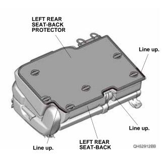
Lift the left rear seat-back protector, and attach masking tape to the left rear seat-back where the snaps will be located.
