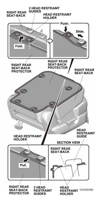
23. Line up the right rear seat-back protector with the right rear seat-back as shown.
