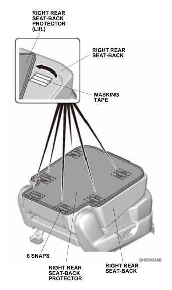
25. Using a T-pin, pierce the right rear seat-back through the hole on the right rear seat-back protector snap as shown. Remove the masking tape attached in step 20 from the right rear seat-back protector. NOTE: Make sure to pierce the right rear seat-back perpendicular. Do not remove the masking tape where the right rear seat-back is not marked yet.
