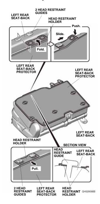
5. Line up the left rear seat-back protector with the left rear seat-back as shown.
