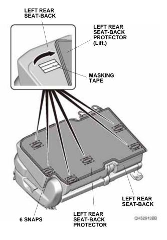
7. Using a T-pin, pierce the left rear seat-back through the hole on the left rear seat-back protector snap as shown. Remove the masking tape attached in step 2 from the left rear seat-back protector.
