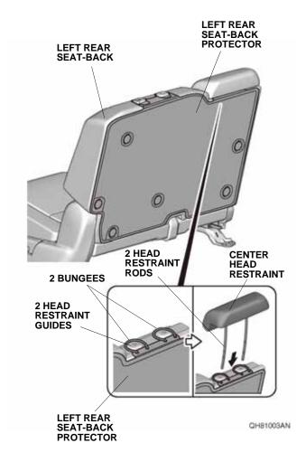
19. Install the head restraint on the left rear seat.
