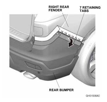
• With the help of an assistant, release the two retaining tabs on each side.
