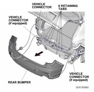
8. Unplug the vehicle connector (if equipped). Then, remove the rear bumper lower cover from the rear bumper.
