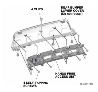
11. Install the hands-free access unit to the rear lower trim with four clips and four self-tapping screws removed in step 10.
