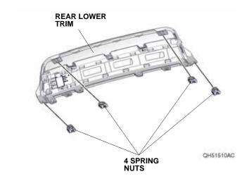
13. Install the rear lower trim to the rear bumper with eight retaining tabs and four bolts removed in step 8. Then, plug the vehicle connector to the hands-free access unit connector (if equipped).
