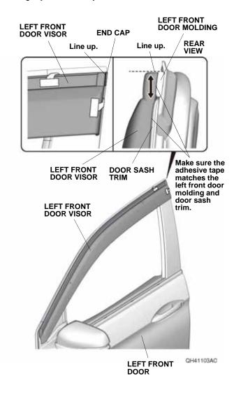
10. While lining up the left front door visor, apply light pressure against the left front door visor as shown.
