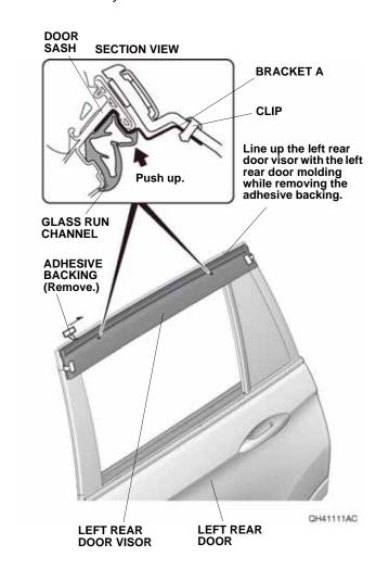
25. Using a rubber roller, apply firm pressure against the left rear door visor and roll from one end to the other. NOTE: Apply firm pressure, especially at the ends.
