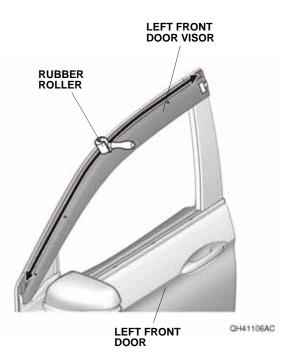
13. While applying light pressure against the left front door visor, carefully remove the taped adhesive backing.
