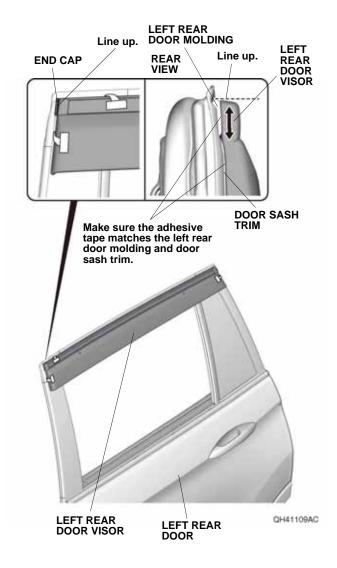
23. While lining up the left rear door visor with the left rear door, apply light pressure against the left rear door visor as shown.
