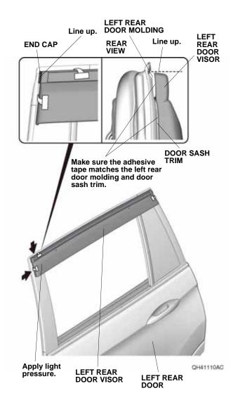
24. While applying light pressure against the left rear door visor, carefully remove the taped adhesive backing as shown. Make sure to push up on the two brackets A while removing the adhesive backing. NOTE: While removing the long top piece of adhesive backing, make sure that left rear door visor is positioned so that the top edge of vehicle chrome is hidden by left rear door visor.
