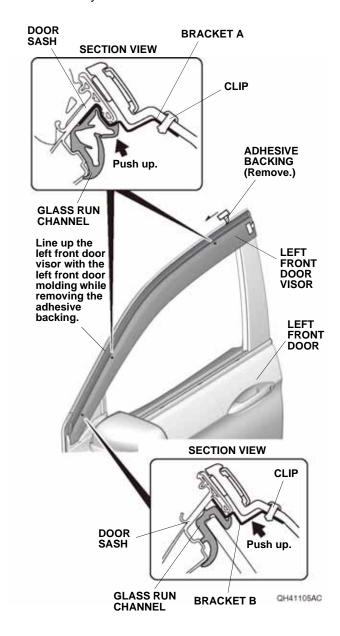
12. Using a rubber roller, apply firm pressure against the left front door visor and roll from one end to the other. NOTE: Apply firm pressure, especially at the ends.
