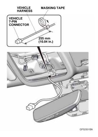
Route the vehicle harness as shown. Be careful not to crease the headliner. Secure the vehicle harness to the holder on the camera cover base, and plug the vehicle 7-pin connector into the automatic day/night mirror.
