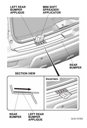
7. Starting from the center and working outward, use the mini soft spreader/applicator to smooth out the left and right sides of the upper section on the left rear bumper applique. Move the mini soft spreader/applicator in one direction only. If you see an air bubble, stop and gently peel up that section to work out the bubble. Work slowly, and keep pressure against the left rear bumper applique.
