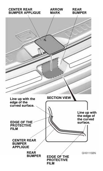
15. Starting from the center and working outward, use the mini soft spreader/applicator to smooth out the center section of the center rear bumper applique. If you see an air bubble, stop and gently peel up that section to work out the bubble. Work slowly, and keep pressure against the center rear bumper applique.
