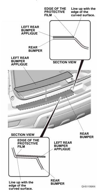
6. Starting from the front and working rearward, use the mini soft spreader/applicator to smooth out the center of the upper section on the left rear bumper applique. Move the mini soft spreader/applicator in one direction only. If you see an air bubble, stop and gently peel up that section to work out the bubble. Work slowly, and keep pressure against the left rear bumper applique.
