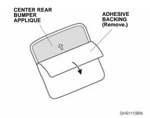
13. Spray the center rear bumper applique with the 3M protective tape application solution.
