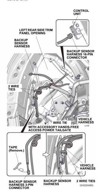
28. Secure the backup sensor harness to the vehicle harness with three wire ties as shown. If the vehicle is equipped withe the accessory hands-free access power tailgate, remove the tape to free the backup sensor harness 3-pin connector. Secure the backup sensor harness to the vehicle harness with two wire ties as shown.
