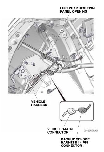
33. Remove the vehicle ground bolt, and secure the backup sensor harness ground terminal to the vehicle ground terminals using that bolt. NOTE: Do not put the ground terminal calkings on top of one another.
