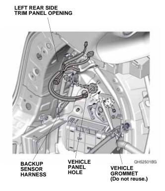
24. Secure the grommet on the backup sensor harness to the vehicle panel hole.
