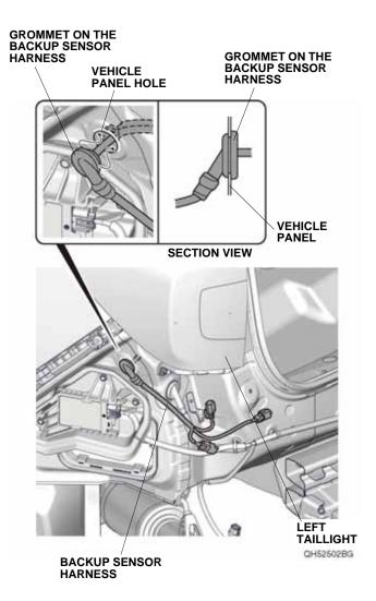
25. Secure the backup sensor harness 6-pin connector to the vehicle bracket as shown.
