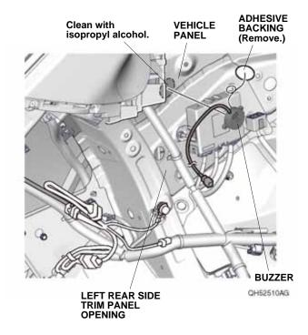
35. Remove the adhesive backing from the buzzer and attach the buzzer to the vehicle panel as shown.
