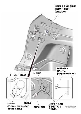
42. While wearing eye protection, drill the pierced mark on the left rear side trim panel with a 3 mm drill bit. Enlarge a 3 mm hole to 26 mm using a 26 mm hole saw. Remove any burrs.
