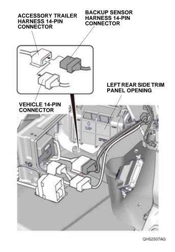
32. Route the vehicle harness, and plug the vehicle 14-pin connector into the backup sensor harness 14-pin connector.
