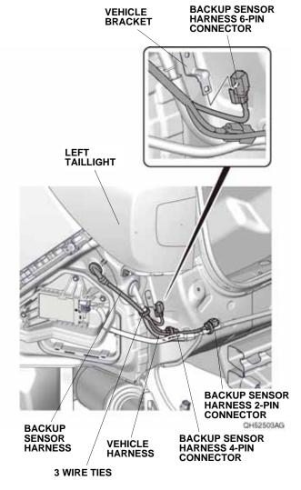
26. Secure the backup sensor harness and backup sensor harness 2-pin and 4-pin connectors to the vehicle harness with three wire ties as shown.
