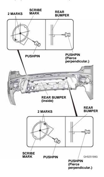
48. While wearing eye protection, drill the 10 pierced marks with a 3 mm drill bit from the inside of the rear bumper.
