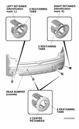
52. Install the two sensors to the left retainer and right retainer.
