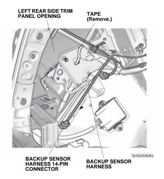
31. Unplug the vehicle 14-pin connector, and plug the backup sensor harness 14-pin connector into the accessory trailer harness 14-pin connector.
