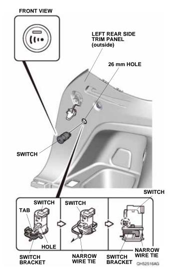
44. Line up the tab on the switch bracket with the hole on the switch and secure the switch bracket to the switch with one narrow wire tie.
