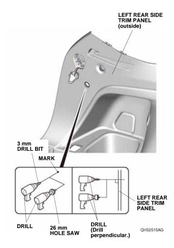
43. Install the switch into the 26 mm hole in the left rear side trim panel.
