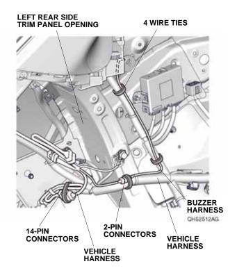
38. Insert the backup sensor harness to the slit on the left rear insulator as shown. Install the left rear insulator.
