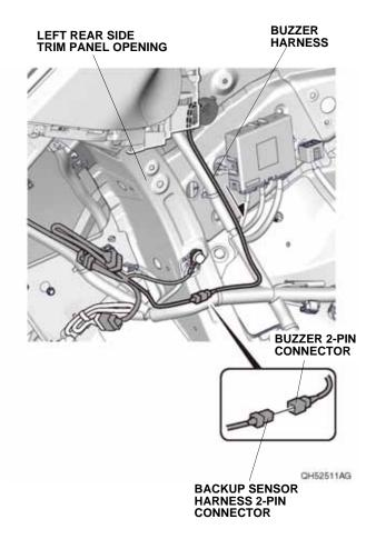
37. Secure the buzzer harness, vehicle harness, 2-pin connectors, and 14-pin connectors to the vehicle harness with four wire ties as shown.
