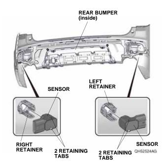
53. Install the two sensors to the two center retainers.
