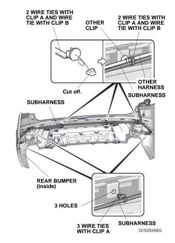
57. Secure the subharness to the rear bumper with three wire ties with clip A as shown.
