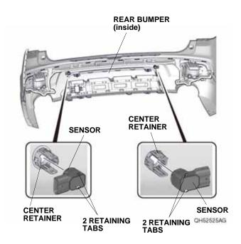
54. Plug the four subharness 6-pin connectors into the four sensors.
