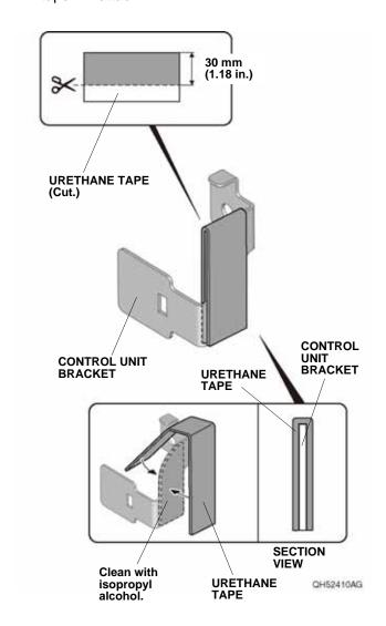
20. Using scissors, cut the urethane tape as shown, and attach a 30 mm (1.18 in.) piece of urethane tape to the control unit bracket as shown.
