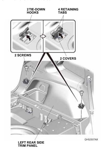
9. Using a plastic trim tool, pull the cover, and remove the cargo hook.
