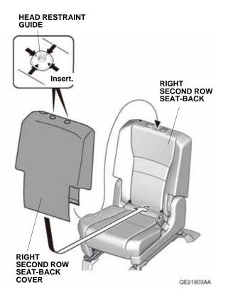
4. Secure the right second row seat-back cover with the fasteners.
