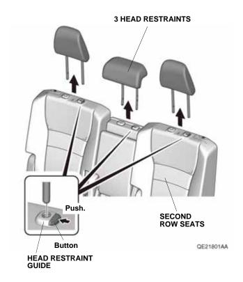
2. Install each head restraint cover on the three head restraints.
