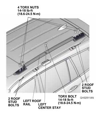
15. Secure the left roof rail to the left center stay with one TORX bolt. Torque the TORX bolt to 14-18 lb-ft (18.6-24.5 N⋅m).
