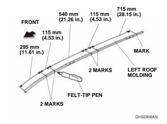
8. While wearing eye protection, use an air saw to cut the molding at the five marks made in step 7. Remove any burrs.
