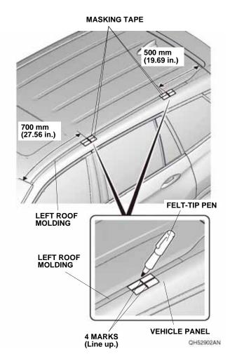
If the roof molding is equipped with a plastic cap, go to step 2; otherwise, go to step 4.
