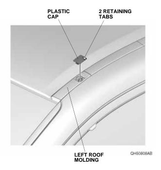
3. Remove the nut from the roof stud bolt.
