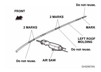
Install the new molding clips to the left roof moldings as shown.
