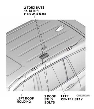
14. Install the left roof rail to the four remaining roof stud bolts with four TORX nuts. Torque the TORX nuts to 14-18 lb-ft (18.6-24.5 N·m).
