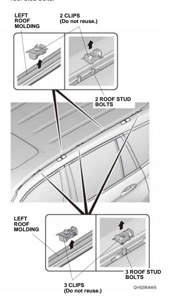
Using a putty knife, remove any excess sealant from the six roof stud bolts.
