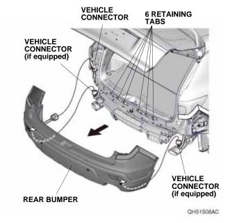
8. Unplug the vehicle connector (if equipped). Then, remove the rear bumper lower cover from the rear bumper.
