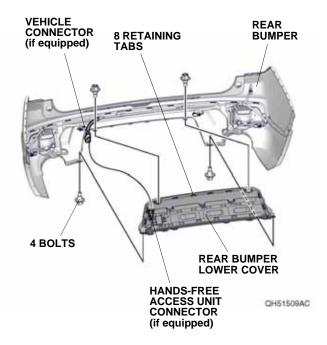
9. Remove the four spring nuts from the rear bumper lower cover.
