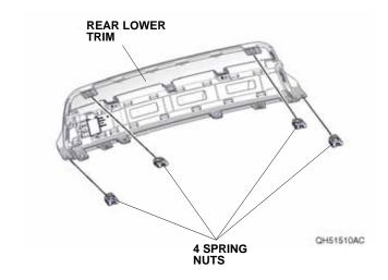
13. Install the rear lower trim to the rear bumper with eight retaining tabs and four bolts removed in step 8. Then, plug the vehicle connector to the hands-free access unit connector (if equipped).
