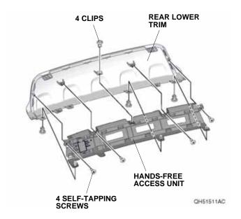
12. Install the four spring nuts removed in step 9 to the rear lower trim.
