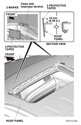
4. Remove the adhesive backing from the two protective tapes, and attach one to the roof panel at each of the two marks you made. Wrap 10 mm (0.39 in.) of protective tape around the lip of the moonroof opening.
