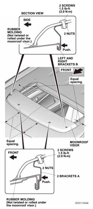
13. Tighten two screws and two nuts on the front of the vehicle first, then tighten two screws and two nuts on each side. Tighten while applying pressure so that there is no gap between the roof panel and the brackets A and B. Torque the screws to 1.5 lb-ft (2.0 N·m).
