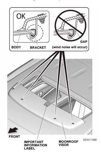
12. Position the moonroof visor with equal spacing on each side. Check that the rubber molding is not twisted or rolled under the moonroof visor.
