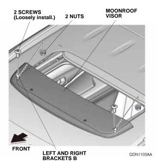
11. Check the information of the IMPORTANT INFORMATION label. To avoid wind noise, install the brackets against the body.
