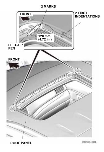
3. Using isopropyl alcohol on a shop towel, clean the roof panel at each of the two marks you have made but do not wipe off the marks.
