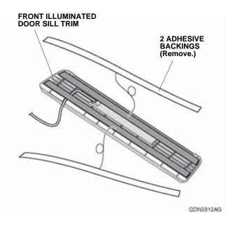
22. Line up the cutout shape on the front illuminated door sill trim with the bump shape on the vehicle panel. Press down firmly on the adhesive part of the front illuminated door sill trim firmly.
