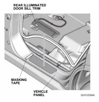
31. While applying light pressure against the rear illuminated door sill trim, carefully remove the taped adhesive backing.
