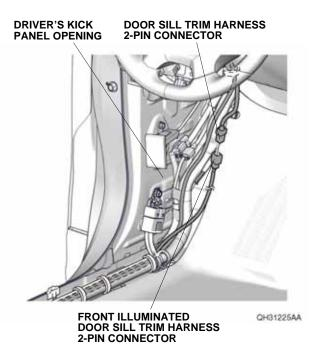
56. Bundle up the excess front illuminated door sill trim harness, and secure it and the 2-pin connectors to the vehicle harness with three wire ties as shown.
