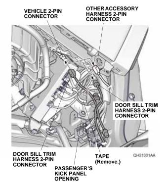
58. Remove the tape to free the door sill trim harness 2-pin connector, and plug it into the other accessory harness 2-pin connector.
