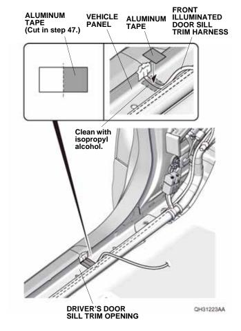
53. Secure the front illuminated door sill trim harness to the vehicle panel with one piece of aluminum tape cut in step 47.
