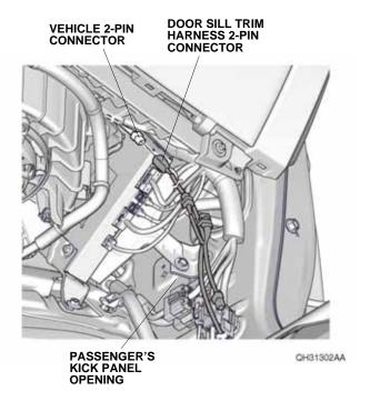
62. Secure the door sill trim harness to the vehicle harness with three wire ties.
