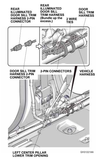
50. Bundle up the excess rear illuminated door sill trim harness, and secure it and the 2-pin connectors to the vehicle harness with two wire ties as shown.
