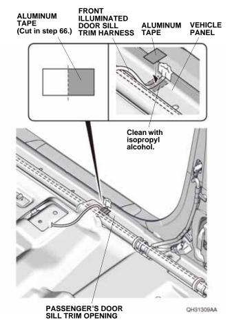
70. Secure the front illuminated door sill trim harness to the vehicle panel with one piece of aluminum tape cut in step 66.
