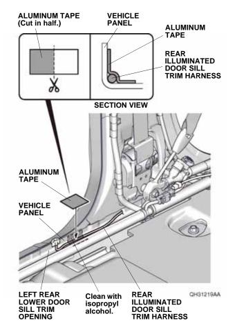
47. Using scissors, cut one aluminum tape in half, and secure the rear illuminated door sill trim harness to the vehicle panel with one piece of aluminum tape as shown.
