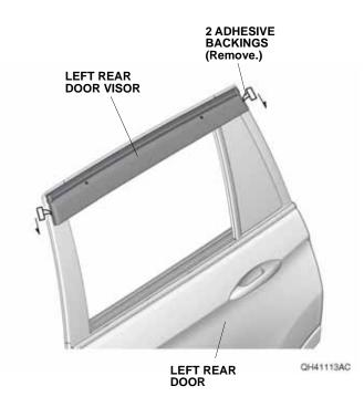
27. Using a rubber roller, apply firm pressure against the left rear door visor and roll from one end to the other. NOTE: Apply firm pressure, especially at the ends.
