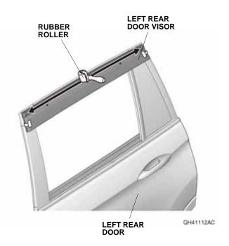
26. While applying light pressure against the left rear door visor, carefully remove the taped adhesive backings.
