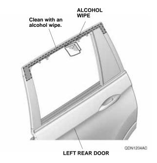
Peel back the adhesive backings, and tape them to the front surface of the left rear door visor with masking tape.
