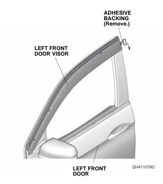
14. Using a rubber roller, apply firm pressure against the left front door visor and roll from one end to the other. NOTE: Apply firm pressure, especially at the ends.
