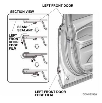
13. Using a shop towel, wipe the 3M protective tape application solution from the left front door edge film. Allow the left front door edge film to dry thoroughly.
