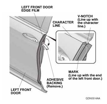
Line up the mark on the left front door edge film with the end of the left front door. While applying light pressure, carefully remove the adhesive backing. Go to step 10.
