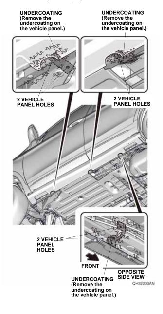
3. Loosely install the left bracket A, left bracket B, and left bracket C to the vehicle panel with six flange bolts.
