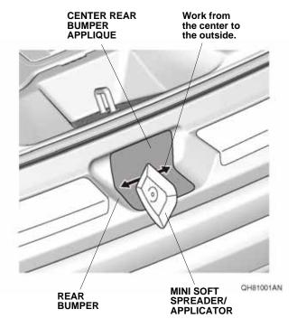
16. Starting from the center and working outward, use the mini soft spreader/applicator to smooth out the center rear bumper applique. If you see an air bubble, stop and gently peel up that section to work out the bubble. Work slowly, and keep pressure against the center rear bumper applique.
