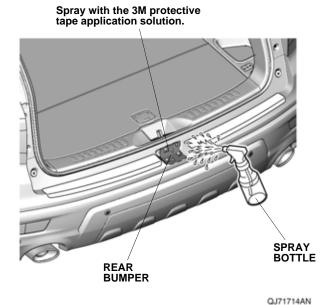
12. Remove the adhesive backing from the center rear bumper applique.
