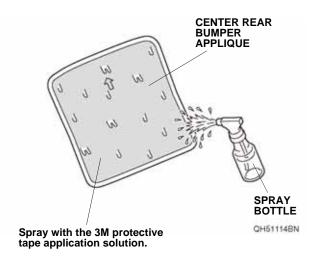
14. Line up the edge of the protective film of the center rear bumper applique with the edge of the curved surface on the rear bumper as shown.
