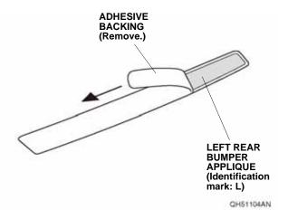
4. Spray the left rear bumper applique with the 3M protective tape application solution.
