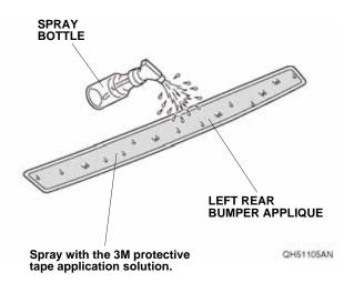
5. Line up the edge of the protective film of the left rear bumper applique with the edge of the curved surface on the rear bumper as shown.
