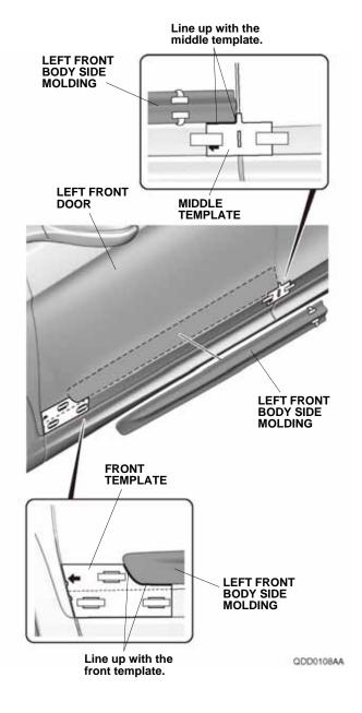
8. While applying light pressure against the left front body side molding, carefully remove the taped adhesive backings.
