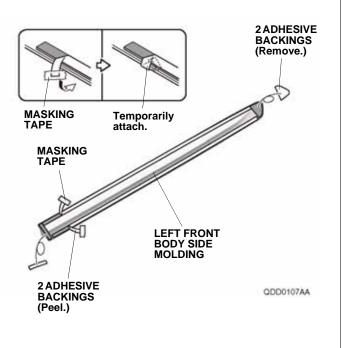
7. Line up the left front body side molding with the front and middle templates, and attach it to the left front door as shown.
