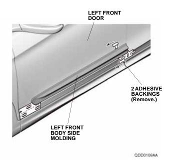
10. Peel back the adhesive backings, and tape them to the front surface of the left rear body side molding with the strips of masking tape. Remove the small piece of adhesive backings.
