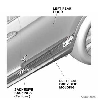
13. Using a rubber roller, apply firm pressure against the left rear body side molding and roll from one end to the other. Apply firm pressure especially at the ends.
