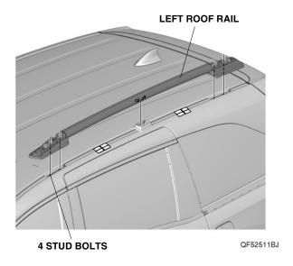
12. Install the four TORX nuts and two TORX bolts. Torque the TORX nuts to 8.9 lb-ft (12 N·m). Install the TORX bolts to 7.4 lb-ft (10 N·m).
