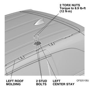
Place the left roof rail over the four remaining stud bolts
