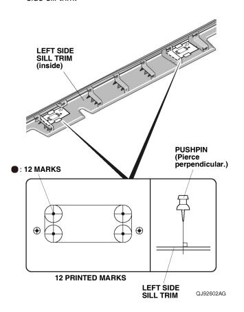
45. While wearing eye protection, drill the 12 pierced marks on the left side sill trim with a 3 mm drill bit. NOTE: Make sure to drill perpendicular to the left side sill trim.
