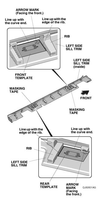
44. Using a pushpin, pierce the inside of the left side sill trim through the center of the 12 printed marks. Remove the front template and rear template. NOTE: Make sure to pierce perpendicular to the left side sill trim.
