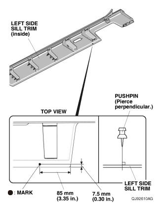
53. While wearing eye protection, drill the pierced mark on the left side sill trim to 7 mm. First drill with a 3 mm drill bit, next with a 6 mm drill bit, and finish with a 7 mm drill bit. Remove any burrs.
