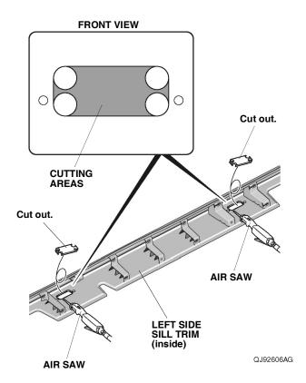
49. Using a pushpin, pierce the inside of the left side sill trim through the center of the four ribs on the left side sill trim
