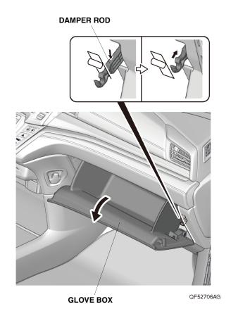
4. Close the glove box, and remove the two bolts.
