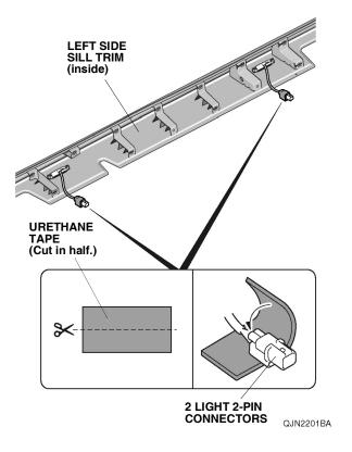
57. Using scissors, cut one urethane tape in half, and wrap one piece of urethane tape around the subharness 2-pin connector as shown.
