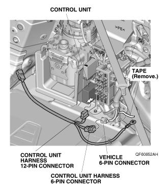
Remove the vehicle ground bolt, and install the control unit harness ground terminal with vehicle ground bolt as shown. Do not put the ground terminal calking on top of one another.
