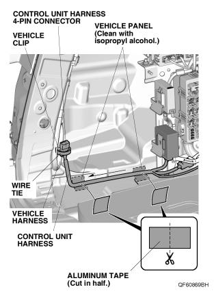
17. Using isopropyl alcohol on a shop towel, thoroughly clean the vehicle panel where the aluminum tape will attach. Using scissors, cut one aluminum tape in half. Secure the control unit harness to the vehicle panel with the two halves of aluminum tape.
