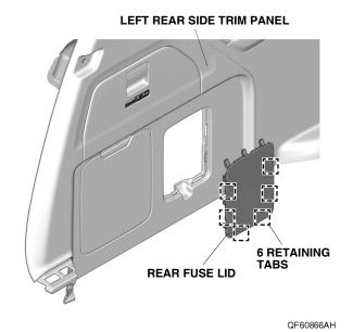
33. Using isopropyl alcohol on a shop towel, thoroughly clean the rear fuse lid where the fuse labels will attach. Attach the fuse labels to the rear fuse lid as shown.
