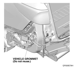
21. Route the socket harness through the vehicle panel hole and secure the grommet on the socket harness into the vehicle panel hole.
