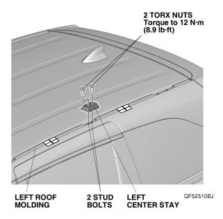
Place the left roof rail over the four remaining stud bolts
