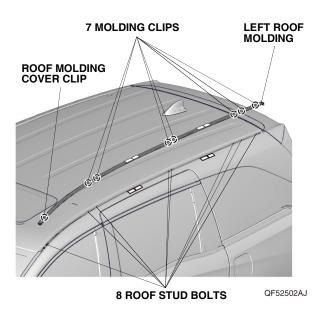
3. Using needle nose pliers, remove the seven molding clips and the roof molding cover clip from either the molding or the roof stud bolts.
