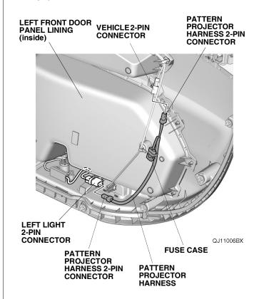
Secure the pattern projector harness to the vehicle harness with one wire tie.
