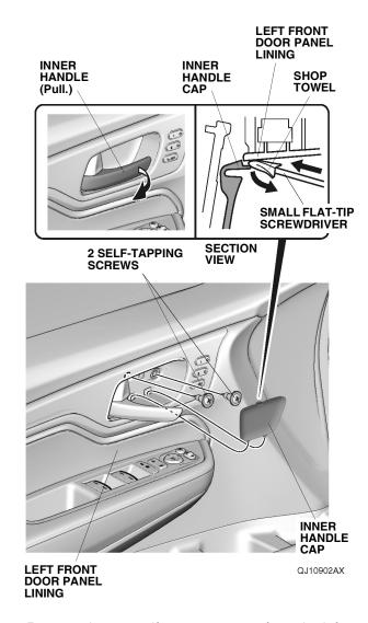
3. Remove the two self-tapping screws from the left front door panel lining.
