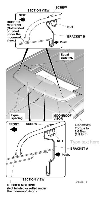
14. Tighten two screws and two nuts on the front of the vehicle first, then tighten two screws and two nuts on each side. Tighten while applying pressure so that there is no gap between the roof panel and the brackets A and B. Torque the screws to 2.0 N·m (1.5 lb·ft).
