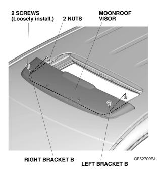
12. Check the information on the IMPORTANT INFORMATION label. To avoid wind noise, install the brackets against the body.
