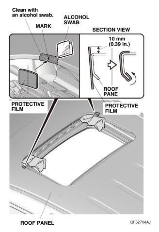
5. Remove the adhesive backing from the two protective films and attach one to the roof panel at each of the two marks you made. Wrap 10 mm (0.39 in.) of protective film around the lip of the moonroof opening.
