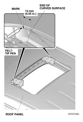
4. Using an alcohol swab, thoroughly clean the roof panel at each of the two marks you have made but do not wipe off the mark.
