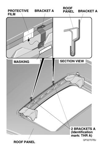
10. Set the moonroof visor on the vehicle roof in front of the moonroof opening, and adjust its position so the holes in the moonroof visor are lined up with the bracket A holes. Loosely install the moonroof visor to the brackets A with two screws and two nuts. Remove the strips of masking tape from the brackets
