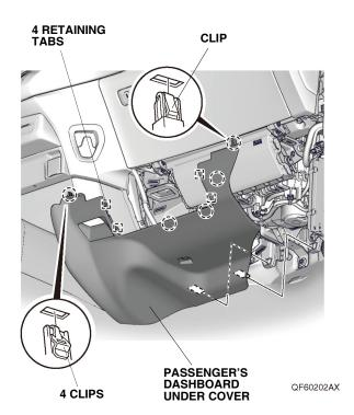
8. Install the ambient light on the passenger's dashboard under cover as shown.
