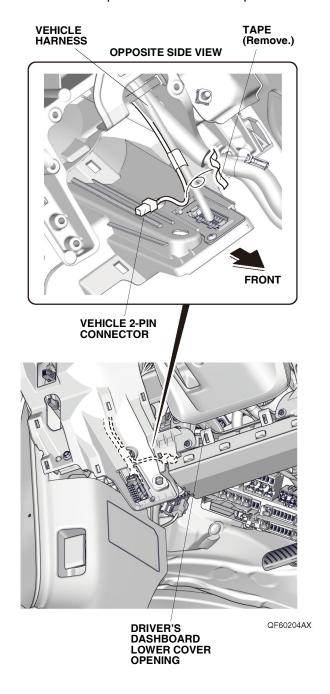
5. Install the ambient light on the instrument panel as shown.
