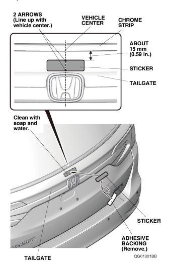
51. Remove the adhesive backing from the sticker. Using the arrows on the sticker, center it about 15 mm (0.59 in.) below the chrome strip and attach it to the tailgate.
