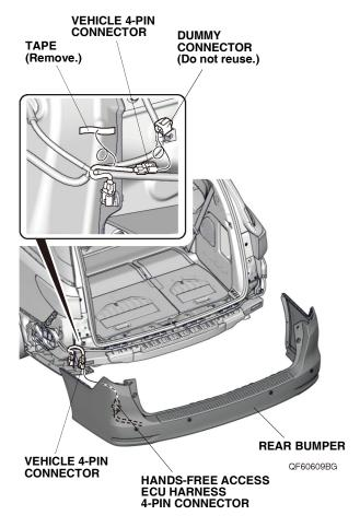
38. With the help of an assistant, bring the rear bumper close to the vehicle, and plug the Hands-Free Access ECU harness 4-pin connector into the vehicle 4-pin connector. Install the rear bumper. Go to step 43.
