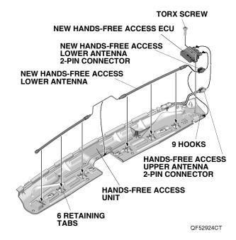
28. Install the new Hands-Free Access lower antenna on the Hands-Free Access unit, and plug the new Hands-Free Access lower antenna 2-pin connector into the new Hands-Free Access ECU.
