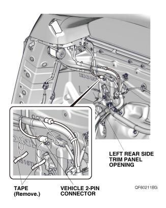
11. Plug the vehicle 2-pin connector into the Hands-Free Access harness 2-pin connector.
