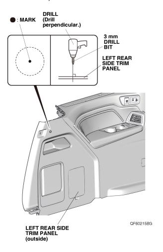
While wearing eye protection, enlarge the 3 mm hole to 26 mm using a 26 mm hole saw. Remove any hurrs
