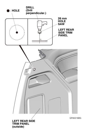
21. Install the switch into the 26 mm hole in the left rear side trim panel.
