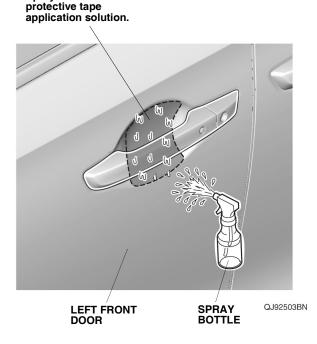
Remove the adhesive backing from the door handle film.
