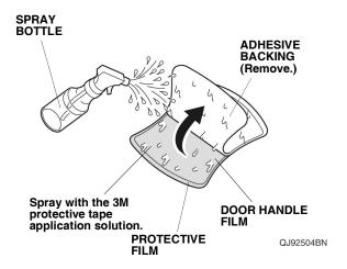
4. Spray the door handle film and protective film with the 3M protective tape application solution.
