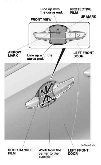
Starting from the center and working outward, use the mini soft spreader/applicator to smooth out the door handle film. If you see an air bubble, stop and gently peel up that section to work out the bubble. Work slowly and keep pressure against the door handle film. 7. Remove the protective film from the door handle film. Using a shop towel, wipe up the 3M protective tape application solution. Allow the door handle film to dry thoroughly.
