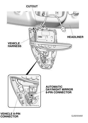
9. Plug the vehicle 8-pin connector into the automatic day/night mirror 8-pin connector.
