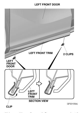
Using a rubber roller, apply firm pressure against the left front trim and roll from one end to the other. Apply firm pressure, especially at the ends.
