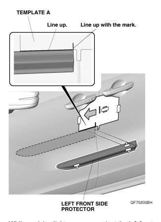
While applying light pressure against the left front side protector, carefully remove the taped adhesive backings.
