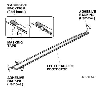
12. Line up the left rear side protector with template A and template B, and install the left rear side protector on the left sliding door.
