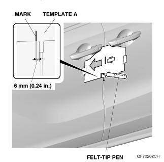
8. Line up the left front side protector with the mark and template A, and install the left front side protector on the left front door.
