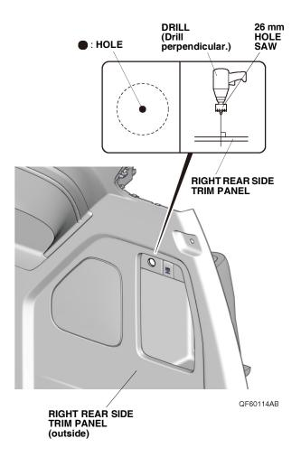
50. Install the switch into the 26 mm hole in the right rear side trim panel.
