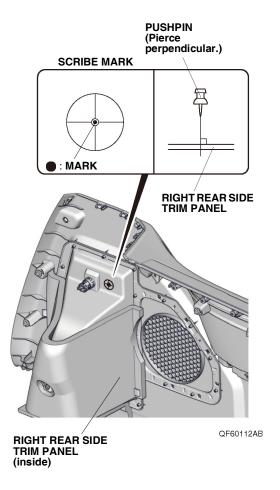
48. While wearing eye protection, drill the pierced mark on the right rear side trim panel with a 3 mm drill bit. NOTE: Make sure to drill perpendicular to the right rear side trim panel.
