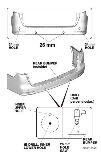
38. Insert the left corner sensor (white) and center sensor (blue) to the rear bumper.
