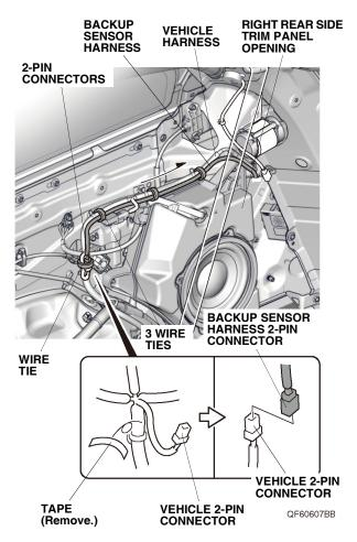
23. Route the backup sensor harness along the vehicle harness, and secure it to the vehicle harness with three wire ties.
