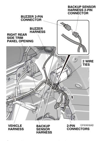
Secure the 2-pin connectors, backup sensor harness, and buzzer harness to the vehicle harness with two wire ties.
