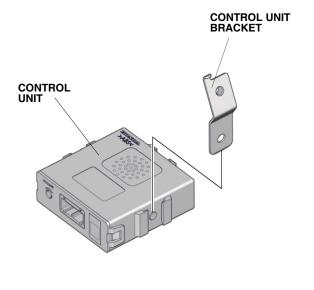
Install the control unit to the vehicle panel with one washer-bolt.
