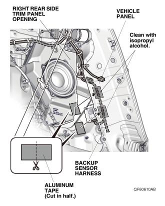
29. Using scissors, cut one piece of aluminum tape in half, and secure the backup sensor harness to the vehicle panel with two halves of aluminum tape as shown.
