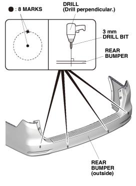
36. While wearing eye protection and drilling from painted side of the rear bumper, enlarge the left outer lower 3 mm hole and right outer lower 3 mm hole to 24 mm using a 24 mm hole saw.
