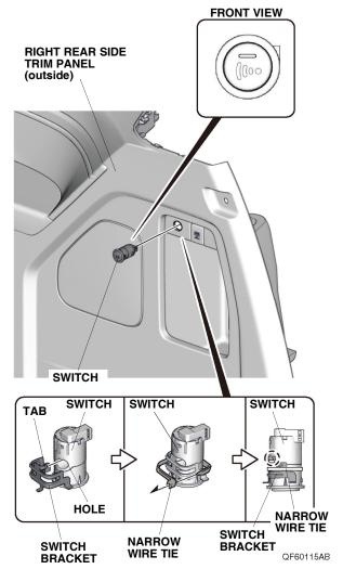
51. Line up the tab on the switch bracket with the hole on the switch and secure the switch bracket to the switch with one narrow wire tie.
