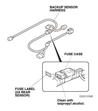
22. Remove the tape to free the vehicle 2-pin connector. Plug the vehicle 2-pin connector into the backup sensor harness 2-pin connector, and secure the 2-pin connectors to the vehicle harness with one wire tie.
