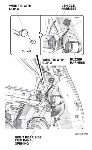
19. Secure the buzzer harness to the vehicle harness with that wire tie. Go to step 21.
