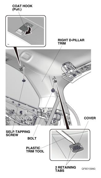
11. Using the plastic trim tool, open the cover and remove the bolt.
