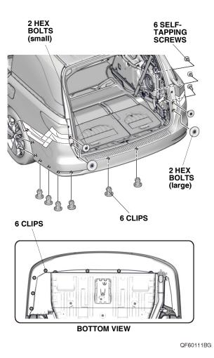
• With the help of an assistant, release the nine retaining tabs on each side.
