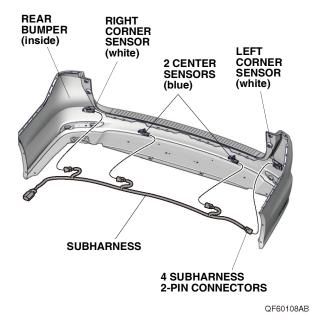
43. Secure the subharness to the rear bumper, left corner sensor clip, and two center sensor clips with three wire ties and two wire ties clip B as shown.
