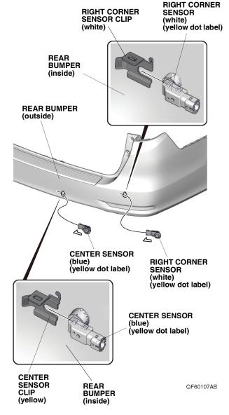
41. Secure the right corner sensor (white) and center sensor (blue) with the right corner sensor clip (white) and center sensor clip (yellow) as shown.
