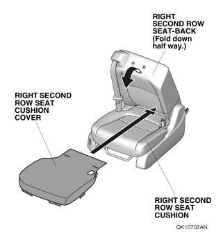
Secure the right second row seat cushion cover to the right second row seat cushion with four tabs and two fasteners.
