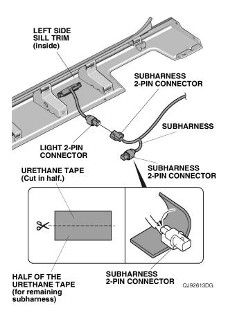
58. Plug the light 2-pin connector into the subharness 2-pin connector.
