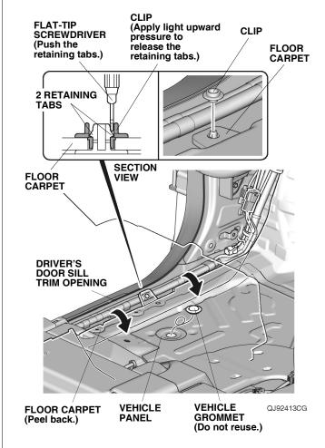
40. Route the puddle light harness as shown, and install the grommet on the puddle light harness to the vehicle panel hole.
