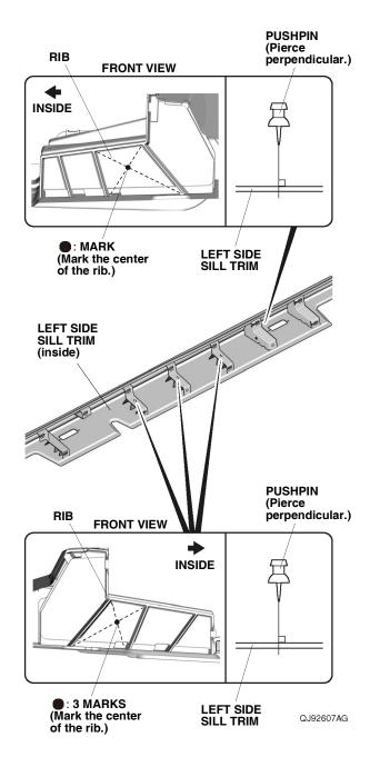
50. While wearing eye protection, drill the four pierced marks on the left side sill trim with a 3 mm drill bit. NOTE: Make sure to drill perpendicular to the left side sill trim.
