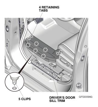
11. Pull away the door opening seal, and remove the driver's kick panel.
