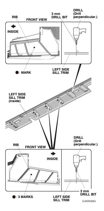
51. While wearing eye protection, enlarge the 3 mm holes on the left side sill trim with a 20 mm hole saw. Remove any burrs.
