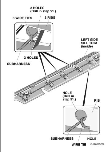
65. Install the 10 clips removed in step 17 to the left side sill trim.
