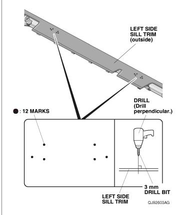
46. While wearing eye protection, enlarge four of the 3 mm holes on the left side sill trim with a 6 mm drill bit. Remove any burrs.
