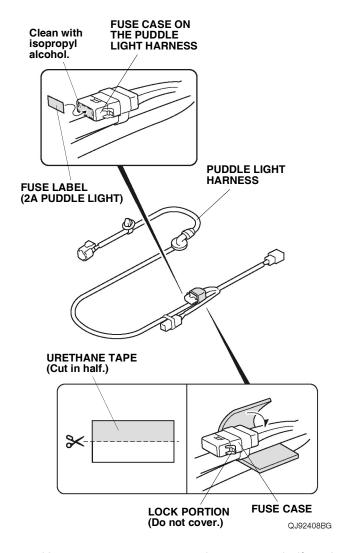
22. Using scissors, cut one urethane tape in half, and wrap one piece around the fuse case as shown.
