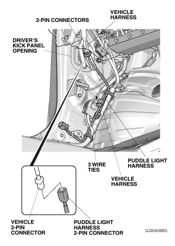
26. Route the puddle light harness along the vehicle harness, and secure it to the vehicle harness with two wire ties.
