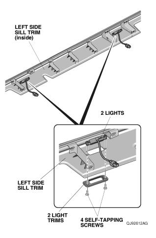
56. Using scissors, cut one urethane tape in half, and wrap one piece of urethane tape around each light 2-pin connector as shown.
