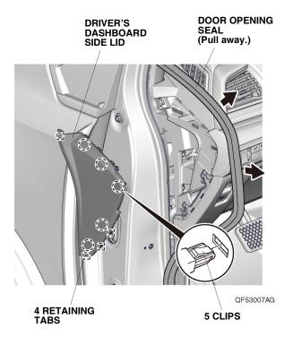
9. Remove the driver's dashboard lower cover, and unplug the vehicle connectors.
