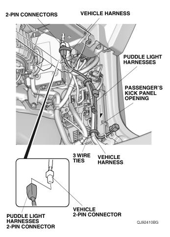
28. Route the puddle light harness along the vehicle harness, and secure it to the vehicle harness with two wire ties. Go to step 39.
