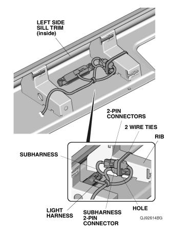
60. Secure the subharness to the light harness with one wire tie as shown.
