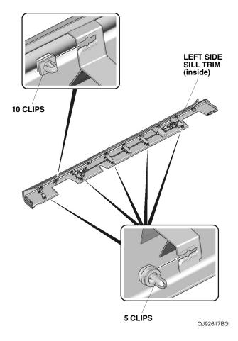
66. Install the five clips removed in step 18 to the left side sill trim.
