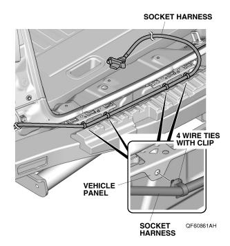
27. Route the socket harness behind the trailer hitch as shown.
