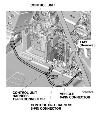
Remove the vehicle ground bolt, and install the control unit harness ground terminal with vehicle ground bolt as shown. Do not put the ground terminal calking on top of one another.
