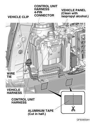
15. Using isopropyl alcohol on a shop towel, thoroughly clean the vehicle panel where the aluminum tape will attach. Using scissors, cut one aluminum tape in half. Secure the control unit harness to the vehicle panel with the two halves of aluminum tape. Go to
