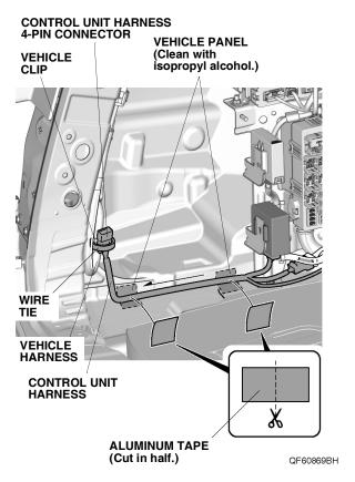
17. Using isopropyl alcohol on a shop towel, thoroughly clean the vehicle panel where the aluminum tape will attach. Using scissors, cut one aluminum tape in half. Secure the control unit harness to the vehicle panel with the two halves of aluminum tape.
