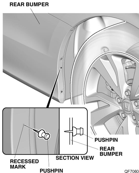
14. Pull apart the rear bumper and the right rear inner fender. Install one grommet on the vehicle panel hole.
