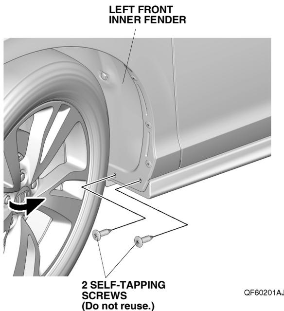
2. Remove the two self-tapping screws from the left front inner fender.
