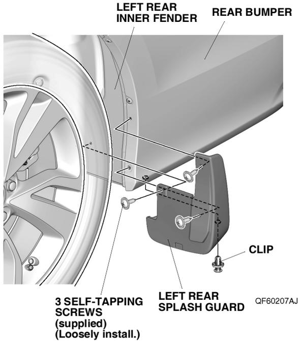
11. Secure the left rear splash guard with the three self-tapping screws in the order shown below. NOTE: Make sure there is no gap between the left rear splash guard and the bumper. If there is a gap, loosen the self-tapping screws, hold the splash guard against the bumper, and retighten the screws.
