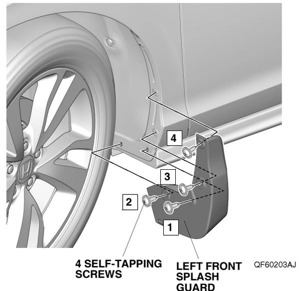
5. Turn the steering wheel fully clockwise, and repeat steps 2 through 4 for the right side of the vehicle.
