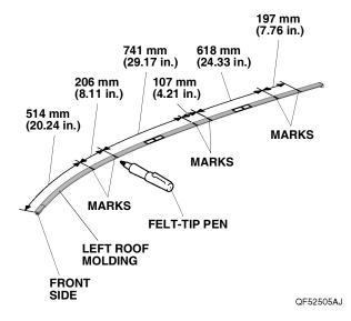
6. While wearing eye protection, use an air saw to cut the molding at the marks made in step 5. Remove any burrs.
