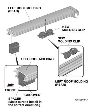
Install the left roof moldings back onto the roof of the vehicle as shown.
