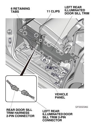
40. Install the left rear illuminated door sill trim on the vehicle panel.
