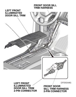
42. Using scissors, cut one piece of urethane tape in half, and attach the two halves of urethane tape to the 2-pin connectors as shown.
