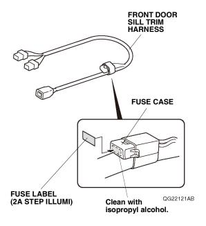
Plug the vehicle 2-pin connector into the front door sill trim harness 2-pin connector, and secure the 2-pin connectors to the vehicle harness with one wire tie.
