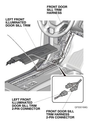
22. Using scissors, cut the urethane tape as shown. Wrap the urethane tape around the 2-pin connectors.
