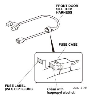
47. Plug the vehicle 2-pin connector into the front door sill trim harness 2-pin connector, and secure the 2-pin connectors to the vehicle harness with one wire tie.
