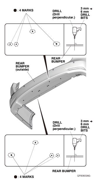
32. While wearing eye protection and drilling from outside of the rear bumper, enlarge four 6 mm holes, with a 9 mm drill bit, then finish with an 11 mm drill bit.
