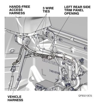
18. Using a pushpin, pierce the center of the scribe mark on the left rear side trim panel.
