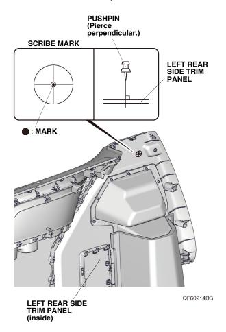
19. While wearing eye protection, drill the pierced mark on the left rear side trim panel with a 3 mm drill bit. NOTE: Make sure to drill perpendicular to the left rear side trim panel.
