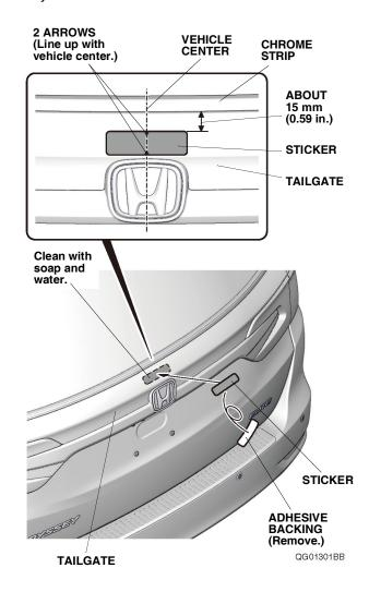
51. Remove the adhesive backing from the sticker. Using the arrows on the sticker, center it about 15 mm (0.59 in.) below the chrome strip and attach it to the tailgate.
