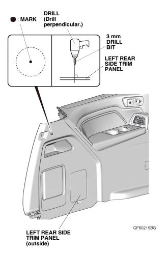
20. While wearing eye protection, enlarge the 3 mm hole to 26 mm using a 26 mm hole saw. Remove any burrs
