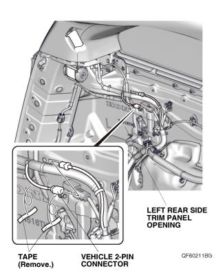
11. Plug the vehicle 2-pin connector into the Hands-Free Access harness 2-pin connector.
