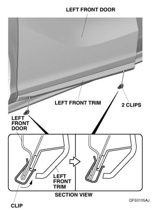
6. Using a rubber roller, apply firm pressure against the left front trim and roll from one end to the other. Apply firm pressure, especially at the ends.
