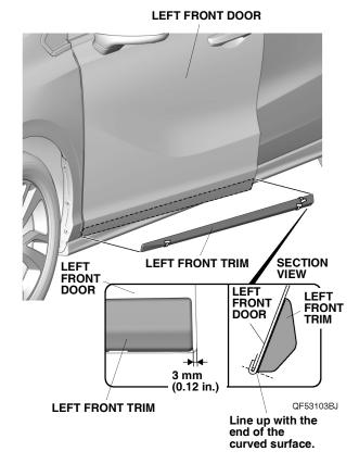
4. While applying light pressure against the left front trim, carefully remove the taped adhesive backings.
