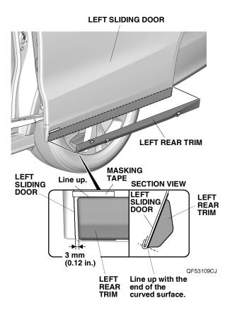
12. While applying light pressure against the left rear trim, carefully remove the taped adhesive backings.
