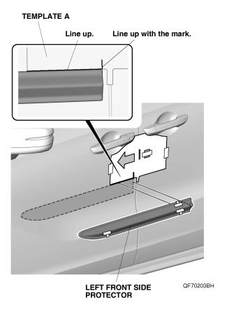
9. While applying light pressure against the left front side protector, carefully remove the taped adhesive backings.
