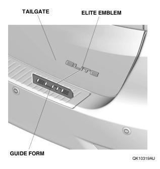
23. Attach the masking tape along the guide form as shown.
