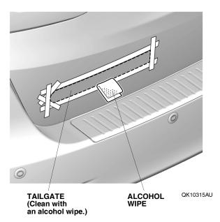
18. Remove the adhesive backing from the ODYSSEY emblem. Line up the guide form with masking tape, and attach the ODYSSEY emblem to the tailgate.
