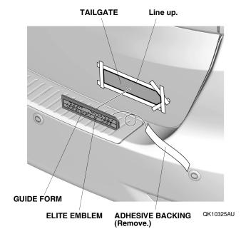
29. Remove the guide form and using the palm of your hand, firmly press the ELITE emblem against the tailgate.
