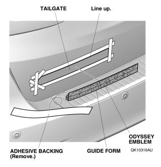
Remove the guide form and using the palm of your hand, firmly press the ODYSSEY emblem against the tailgate.
