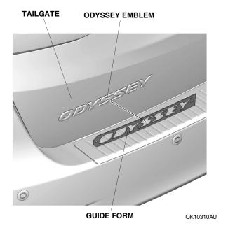
13. Attach the masking tape along the guide form as shown.
