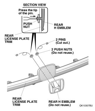
8. Using an alcohol wipe, thoroughly clean the rear license plate trim where the rear H emblem will attach.
