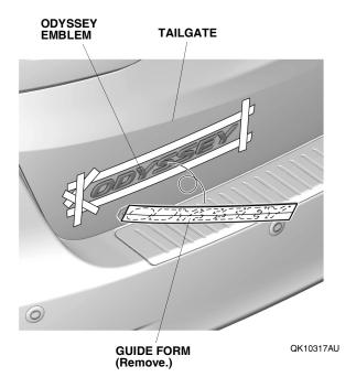
20. Remove the masking tape from the tailgate.
