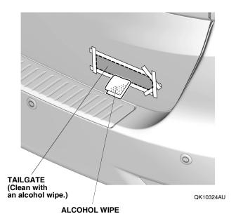
28. Remove the adhesive backing from the ELITE emblem. Line up the guide form with masking tape, and attach the ELITE emblem to the tailgate.
