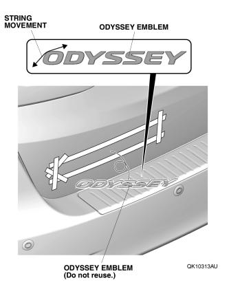
16. Install the ODYSSEY emblem in the guide form, and temporarily secure it with masking tape.
