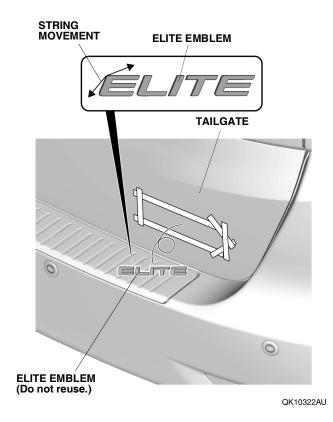
26. Install the ELITE emblem in the guide form, and temporarily secure it with masking tape.
