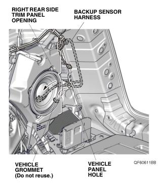
31. Secure the grommet on the backup sensor harness into the vehicle panel hole.
