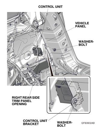
16. Using isopropyl alcohol on a shop towel, thoroughly clean the vehicle panel where the buzzer will attach.
