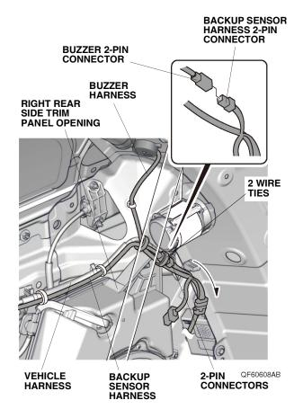
25. Secure the 2-pin connectors, backup sensor harness, and buzzer harness to the vehicle harness with two wire ties.
