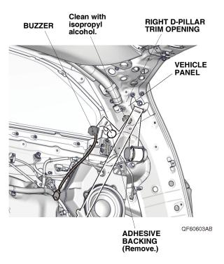
17. Remove the adhesive backing from the buzzer, and attach the buzzer to the vehicle panel as shown.
