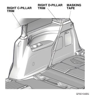
6. Using the plastic trim tool, open the two covers and remove the two self-tapping screws.
