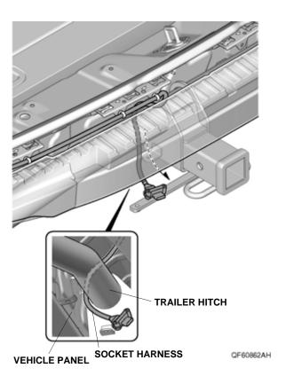
28. Secure the socket harness 4-pin connector to the trailer hitch with two flange bolts.
