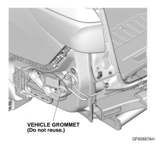
21. Route the socket harness through the vehicle panel hole and secure the grommet on the socket harness into the vehicle panel hole.
