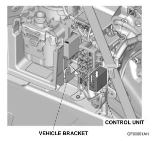
11. Remove the tape from the vehicle 6-pin connector and plug the vehicle 6-pin connector into the control unit harness 6-pin connector. Plug the control unit harness 12-pin connector into the control unit.
