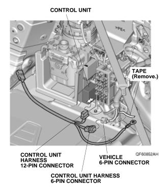
12. Remove the vehicle ground bolt, and install the control unit harness ground terminal with vehicle ground bolt as shown. Do not put the ground terminal calking on top of one another.
