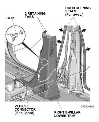
11. Pull away the door opening seal, and remove the driver's dashboard side lid.
