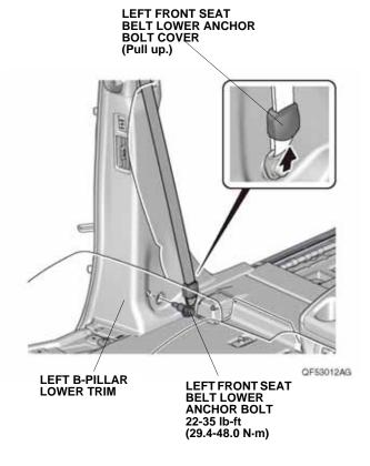
17. Pull away the door opening seals, and remove the left B-pillar lower trim, and unplug the vehicle connector (if equipped).
