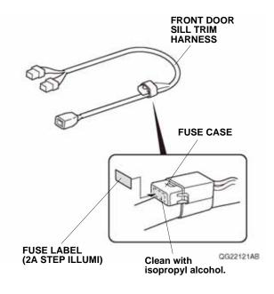
47. Plug the vehicle 2-pin connector into the front door sill trim harness 2-pin connector, and secure the 2-pin connectors to the vehicle harness with one wire tie.
