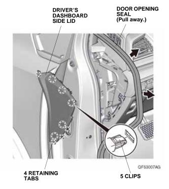
12. Remove the driver's dashboard lower cover, and unplug the vehicle connectors.
