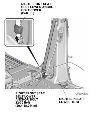
10. Pull away the door opening seals, and remove the right B-pillar lower trim, and unplug the vehicle connector (if equipped).
